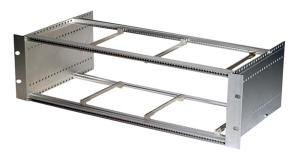
Complete 19" rack with side walls, transversal rails, and mounting flanges. 6 guiding rails are included for set up of a system. The rails shall be fixed to the rack by the included screws (12 screws M2.5 x 12 and 12 nuts).
