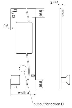
Fig. 5 Intermas system front panels (various case sizes)
